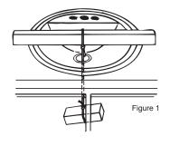
Detach the faucet from the shut-off valves by unscrewing the compression nut at the joints between the valves and the water supply tubes.
